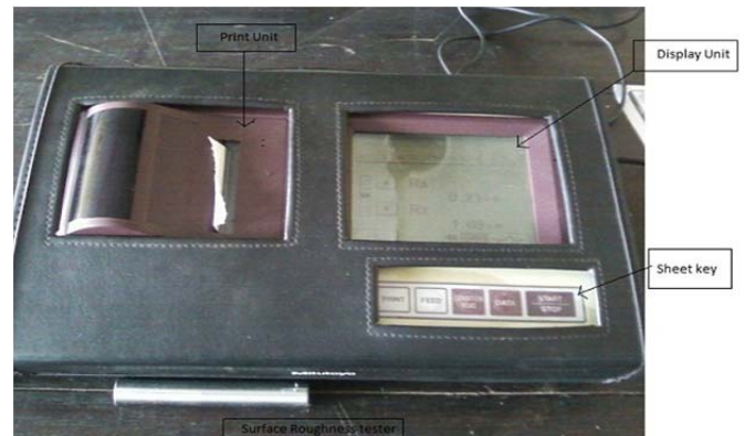
Fig. 3: Mitutoyo Surftest surface roughness tester
